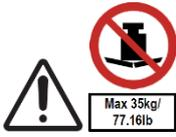
Objects must be placed in the centre of the shelf plate. Observe the maximum load! Do not place any liquids on the shelf plate.
