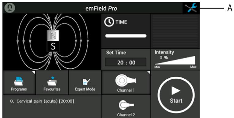
**Selecting configuration** Pressing the Configuration button (A) immediately switches to the configuration menu.
